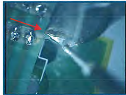
End Position – Tip Location Slide past last pin
