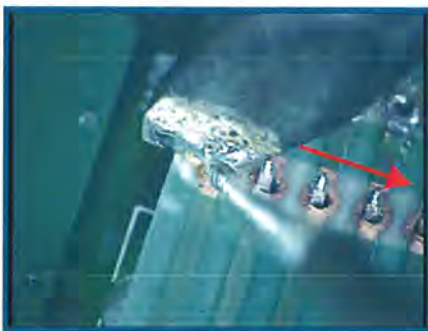
Start Position – Tip Location Iron Tip 50% on past first pin
