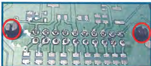
Plastic Snap-Lock Prevents Iron tip from sliding past the last terminal
