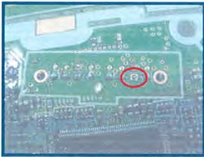
Solder Void Total missed joint, tip may have hit top of terminal
